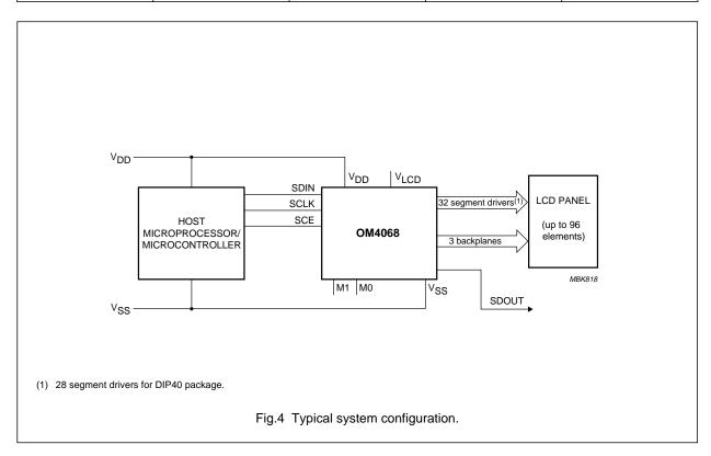
The host microprocessor/microcontroller maintains the 3-line bus communication channel with OM4068. The internal oscillator requires no external components. The appropriate intermediate biasing voltage for the multiplexed LCD waveforms are generated on-chip.
