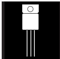
**100V Thru 500V, Up To 14 Amp, N-Channel MOSFET With Or Without Zener Gate Clamp Protection**
