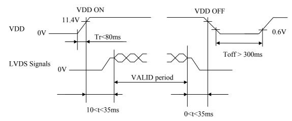
Note1: LVDS signals should be measured at the terminal of  $100\Omega$  resistor.
