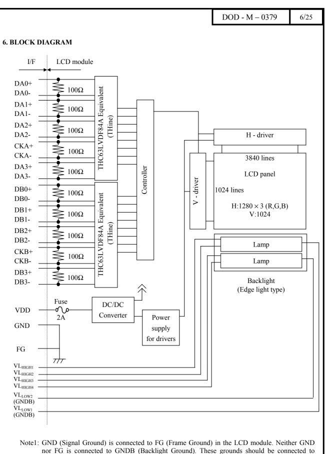
nor FG is connected to GNDB (Backlight Ground). These grounds should be connected to system ground in customer equipment.
