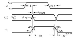
**Figure 4. Driver Timing Measurement**
