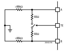
Figure 9. Equivalent Input Resistance into A and B (on the LTC2854, Valid if Driver is Disabled)
