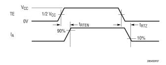
Figure 8. Termination Resistance and Timing Measurements
