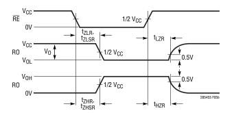
Figure 7. Receiver Enable and Disable Timing Measurements
