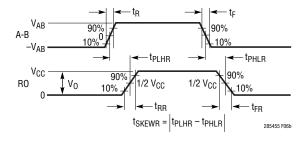
Figure 6. Receiver Propagation Delay Measurements
