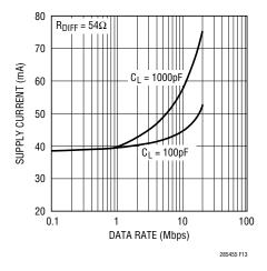
Figure 13. Supply Current vs Data Rate
