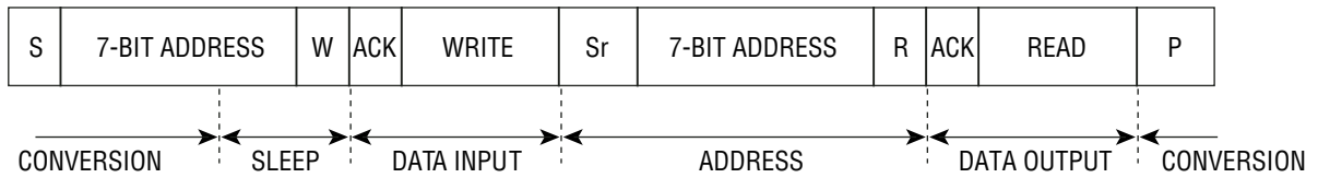
Figure 6. Write, Read, Start Conversion
