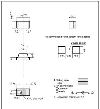
U type: There is Anode mark on the device because polarity faces in the opposite direction.
