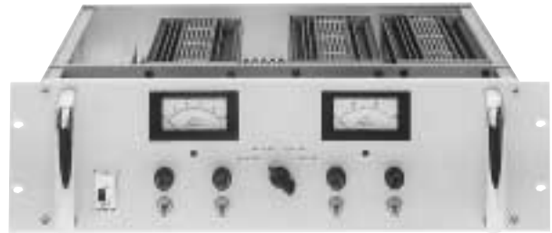
Four outputs, each separately switched, are provided by this 5 1/4" high assembly. The voltmeter and ammeter may be switched to monitor any output.
