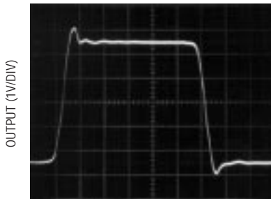
Large-Signal Transient Response ( A_V = 2 )
