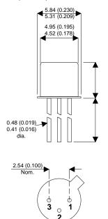
**Bipolar NPN Device in a** Hermetically sealed TO18 Metal Package.
