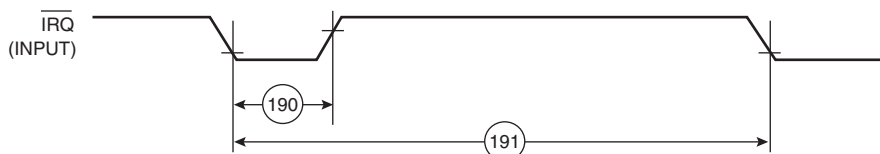
Figure 20. Interrupts Timing Diagram
