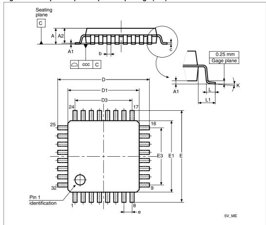
Table 26. 32-pin low profile quad flat package mechanical data
