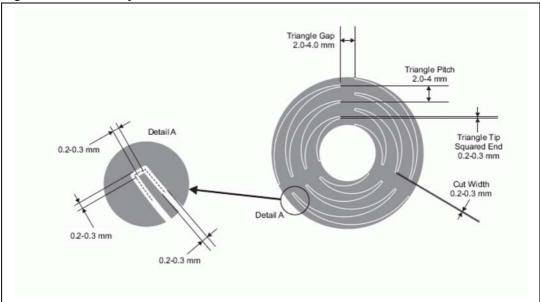
As with touch button electrodes, rotors and sliders can be constructed as etched areas on a PCB or flex circuit, or from clear conductors such as Indium Tin Oxide (ITO) or screen-printed Orgacon™ (Agfa) to allow backlighting effects, or for use over an LCD display.
