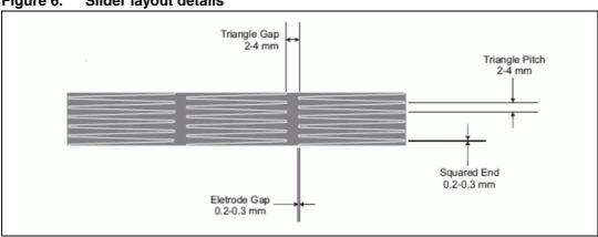
Figure 6. Slider layout details
