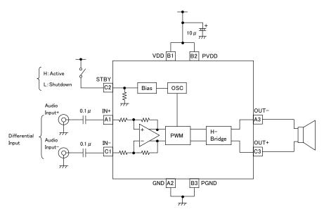
Fig.2 Differential input with coupling input capacitors
