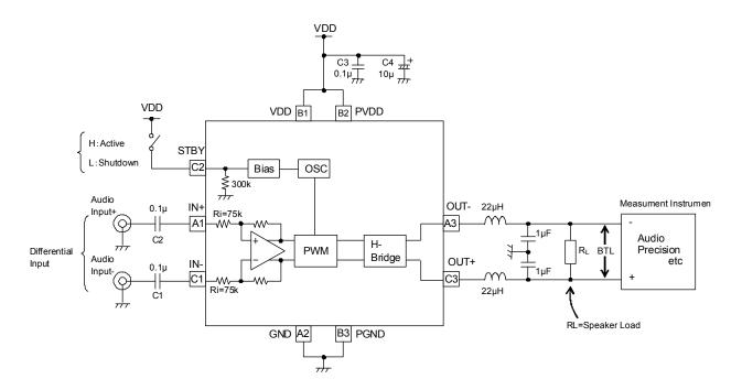
When measuring Audio characteristics, insert LC filter during the output terminal of IC and the speaker load and measure it. Arrange LC filter as close as possible to the output terminal of IC. In case of L= $22\mu H$ , C= $1\mu F$ , the cutoff frequency becomes the following.
