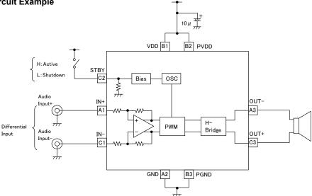
Fig.1 Differential input for mobile phone
