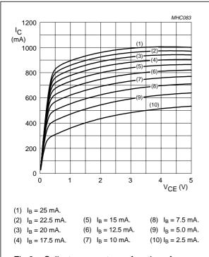
Fig.6 Collector current as a function of collector-emitter voltage; typical values.
