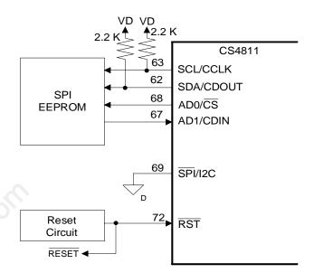
Figure 5. Typical Connection Diagram, SPI Mode
