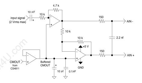
Figure 6. Optional Line Input Buffer
