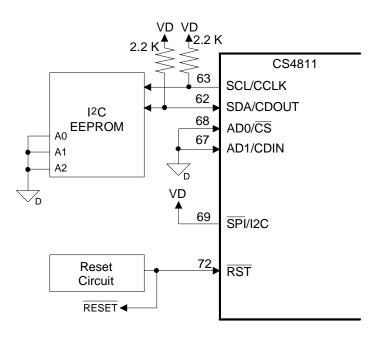
Figure 4. Typical Connection Diagram, I<sup>2</sup>C Mode
