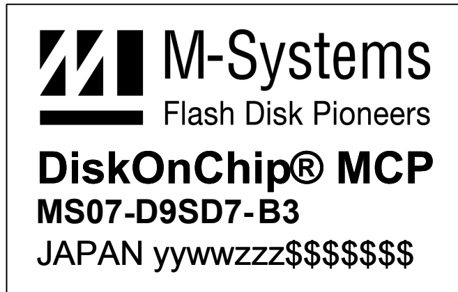
Figure 4: DiskOnChip-Based MCP Product Marking
