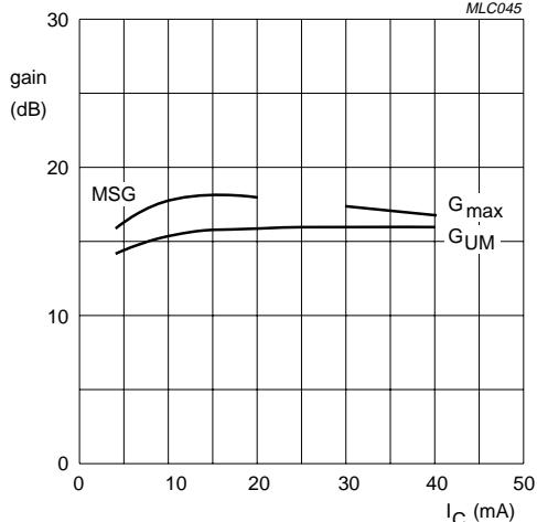
$f = 900 \text{ MHz}; V_{CE} = 8 \text{ V.}$
