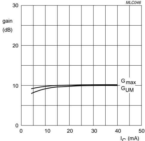
$f = 2 \text{ GHz}; V_{CE} = 8 \text{ V.}$
