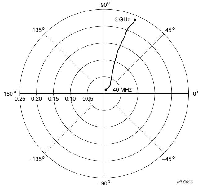
$V_{CE} = 8 \text{ V}; I_C = 40 \text{ mA}.$ Fig.21 Common emitter reverse transmission coefficient ( $s_{12}$ ); typical values.
