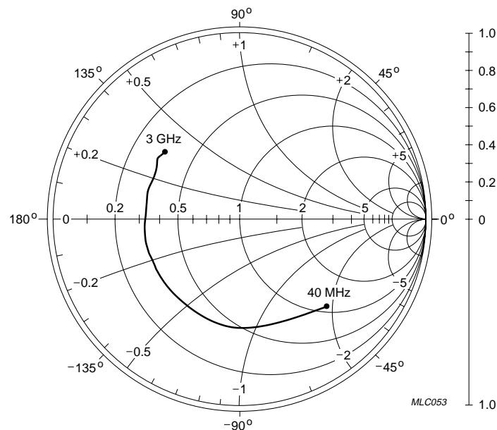
$V_{CE} = 8 \text{ V}; I_C = 40 \text{ mA}; Z_0 = 50 \Omega.$ Fig.19 Common emitter input reflection coefficient ( $s_{11}$ ); typical values.
