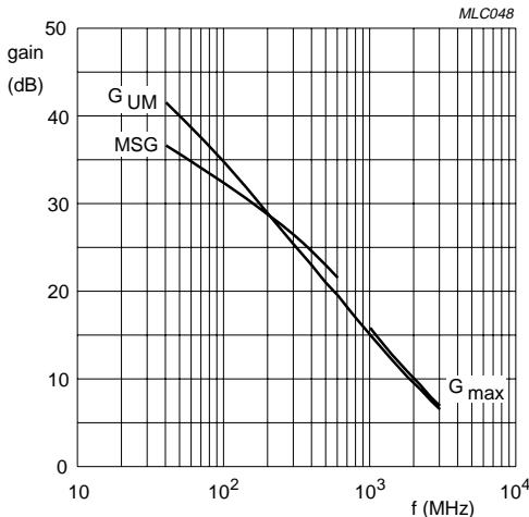
$I_C = 40 \text{ mA}; V_{CE} = 8 \text{ V.}$
