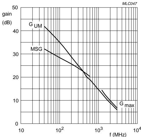
$I_C = 10 \text{ mA}; V_{CE} = 8 \text{ V.}$
