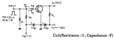
$-10l_{B1}=10l_{B2}=l_{C}=-50mA$  $R_L = 3\,k\,\Omega$  ,  $R_B = 200\,\Omega$  at  $I_C = -50\,m\,A$
