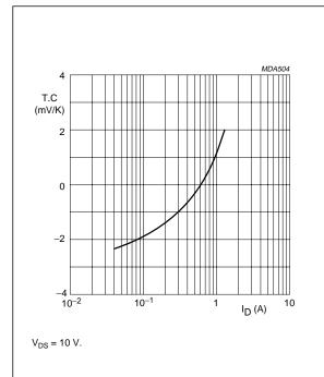
Temperature coefficient of gate-source voltage as a function of drain current, typical values per section.
