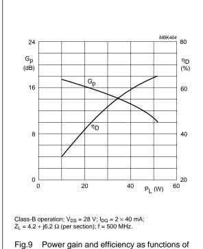
Fig.9 Power gain and efficiency as functions of load power, typical values per section.
