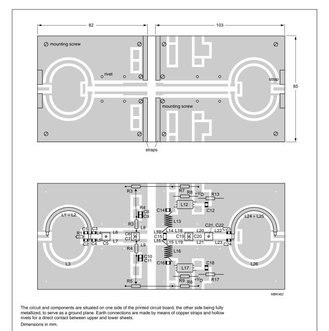
Fig.12 Component layout for 500 MHz class-B test circuit.
