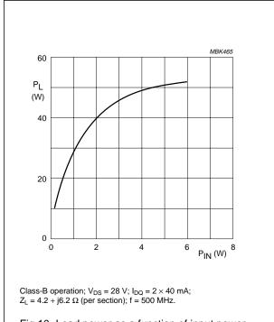
Fig.10 Load power as a function of input power, typical values per section.
