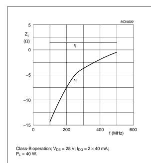
Fig.13 Input impedance as a function of frequency (series components), typical values per section.
