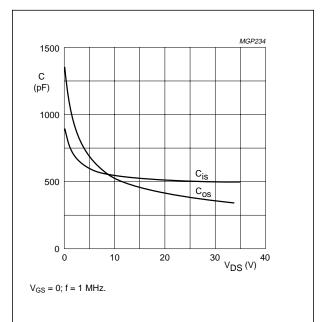
Fig.7 Input and output capacitance as functions of drain-source voltage, typical values per section.
