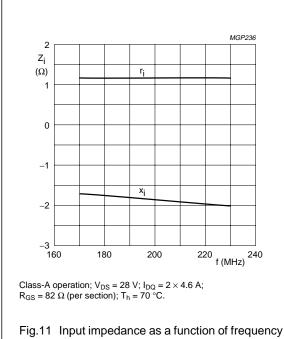
Fig.11 Input impedance as a function of frequency (series components), typical values.
