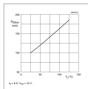
Fig.6 Drain-source on-state resistance as a function of junction temperature, typical values per section.
