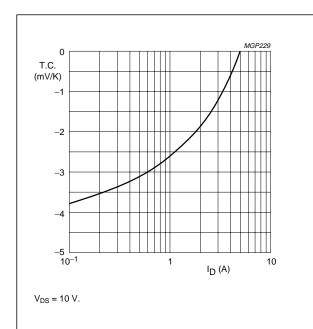
Fig.4 Temperature coefficient of gate-source voltage as a function of drain current, typical values per section.
