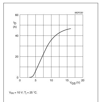
Fig.5 Drain current as a function of gate-source voltage, typical values per section.
