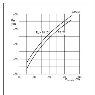
Fig.9 Intermodulation distortion as a function of peak synchronized output power.
