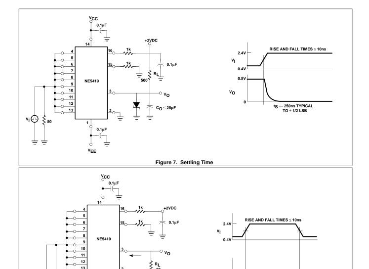
Figure 8. Propagation Delay Time
