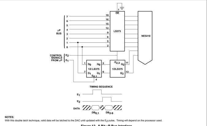
Figure 12. 8-Bit  $\mu P$  Bus Interface
