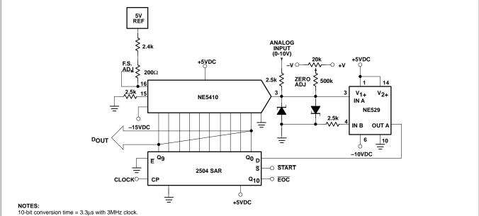
This converter uses a 2504 12-bit successive approximation register in the short cycle operating mode where the end of conversion signal is taken from the first unused bit of the SAR (Q<sub>10</sub>).
