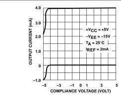
Figure 1. Output Current vs Output Compliance Voltage
