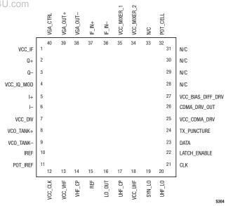
Figure 1. SKY74702 Pinout – 40-Pin RFLGA Package (Top View)
