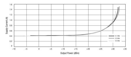
Figure 8. Supply Current vs Output Power, CW Input
