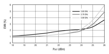
Figure 4. High Band EVM vs Output Power
