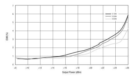
Figure 3. Low Band EVM vs Output Power
