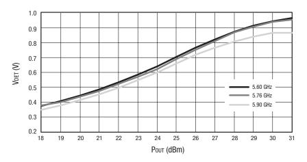
Figure 6. High Band Detector Voltage vs Output Power
