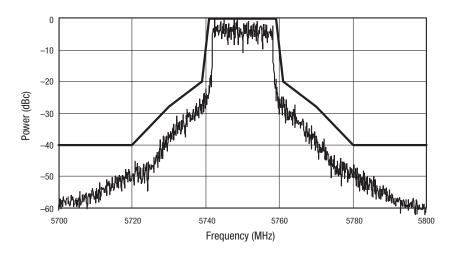
Figure 7. Typical Spectral Response With 802.11a 64-QAM OFDM Signal (Output Power = +27 dBm)
