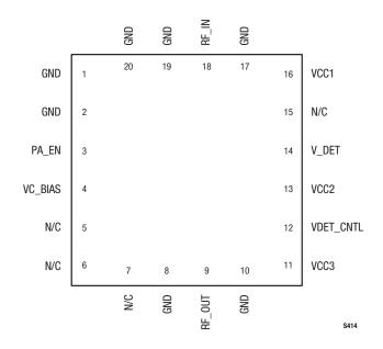
Figure 1. SKY65137 Pinout – 20-Pin MCM (Top View)
