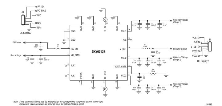
Figure 10. SKY65137 Evaluation Board Schematic
