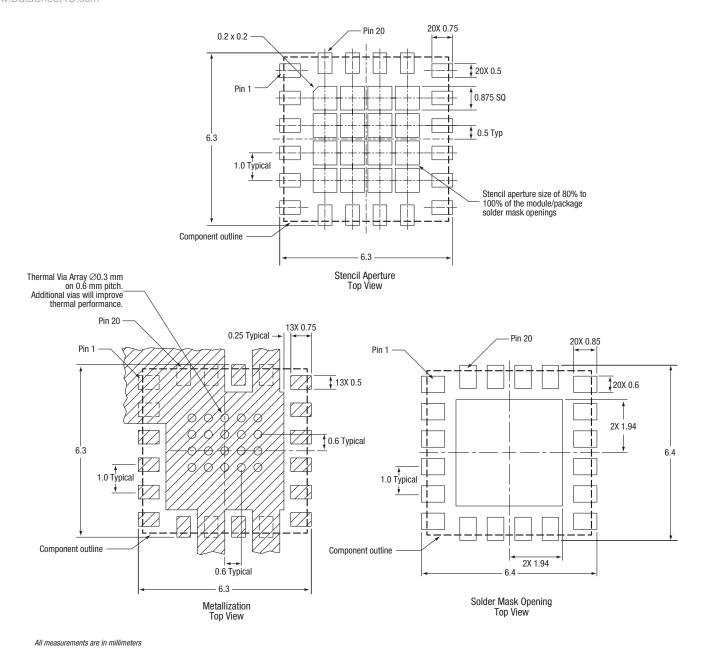
Figure 12. PCB Layout Footprint For The SKY65137
