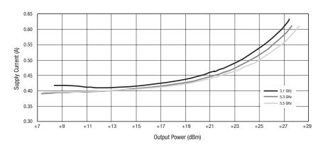
Figure 9. Supply Current vs Output Power, Modulated Input
