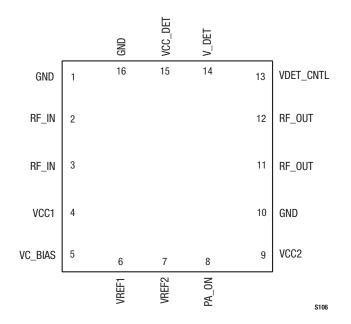
Figure 1. SKY65131 Pinout – 16-Pin MCM (Top View)
