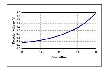
Figure 8. Detector Output Voltage vs RF Output Power
