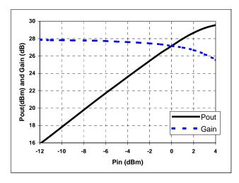
Figure 3. Typical Pout and Gain vs PIN @ 2.442 GHz
