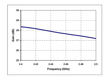
**Figure 4. Typical Gain vs Frequency Response**
