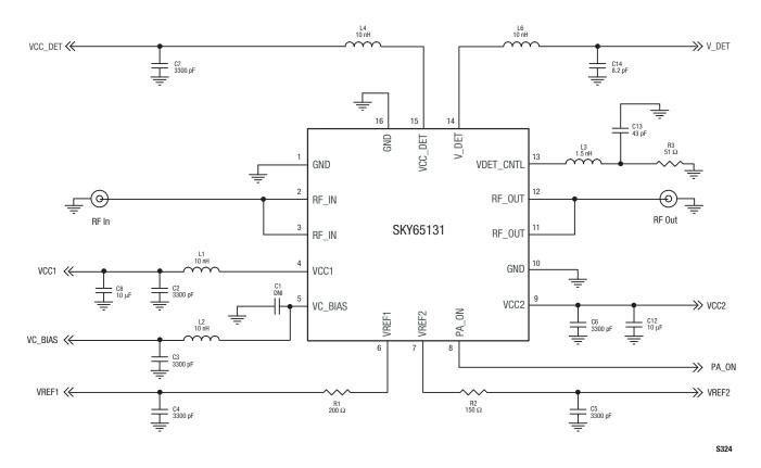
Figure 10. SKY65131 Evaluation Board Schematic
