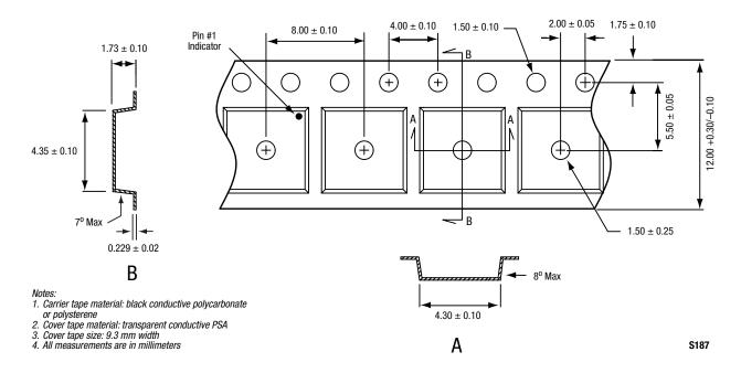
Figure 12. SKY65131 16-Pin MCM Tape and Reel Dimensions
