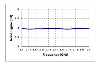
**Figure 5. Typical Noise Figure Performance vs Frequency**
