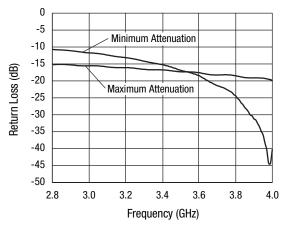
**Output Return Loss vs. Frequency**
