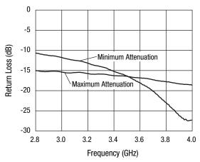
**Input Return Loss vs. Frequency**
