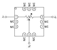
Ground is connected to paddle on bottom.
