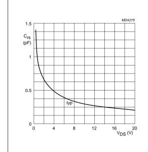
$\begin{aligned} \text{Fig.2} \quad & \text{V}_{\text{GS}} = \text{0 for BF510 and BF511;} \\ & \text{I}_{\text{D}} = \text{5 mA for BF512 and BF513;} \\ & \text{f} = \text{1 MHz; T}_{\text{amb}} = \text{25 °C.} \end{aligned}$
