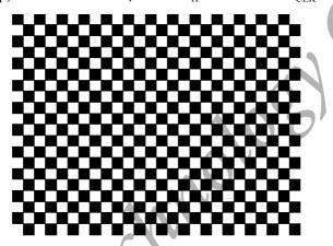
Max value is Black Pattern : 900 line mode. Circuit condition (Max) : VCC= $3.3 \vee f_V=60 \text{ Hz} f_H=55.56 \text{ kHz} \cdot f_{CLK}=48.89 \text{ MHz}$  (one of LVDS dual port).
