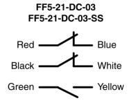
NOTE: Contact configurations show under closed condition for guard device.
