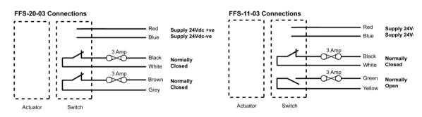
Contact configurations show under closed condition for guard device.
