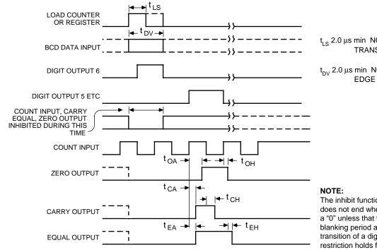
t<sub>LS</sub> 2.0 μs min NOTE: REF. TO POSITIVE TRANSITION OF DIGIT OUTPUT
