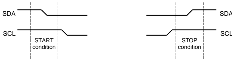
Figure 16-3. START and STOP Conditions
