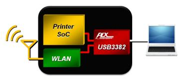
As the successor of the gold standard NET2280 (PCI to USB 2.0 peripheral controller), the USB338x can be used with existing NET228x software with no or minimal change. Driver stacks for the NET228x are already available in common printer OS's such as Linux and VxWorks. Therefore adding USB 3.0 support in an existing driver stack is as easy as adding the hardware by simply plugging the USB338x into the system.
