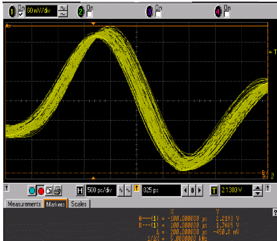
Figure 2. MPC8260 Power Input from a Non-optimized Source
