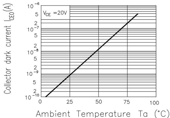
Fig. 3 Relative Collector Current vs. Ambient Temperature
