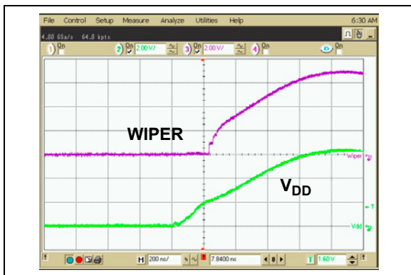
FIGURE 2-15: 2.1 k \Omega – Power-Up Wiper Response Time.
