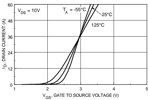
Figure 5. Transfer Characteristics.
