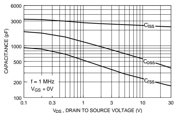
Figure 8. Capacitance Characteristics.
