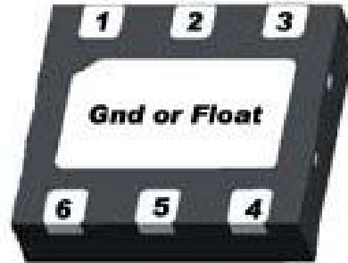
Figure 3. Pin Configuration (Bottom View)
