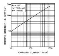
Fig. 4 Emitting strength vs. forward current
