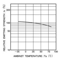
Fig. 5 Relative emitting strength vs. ambient temperature
