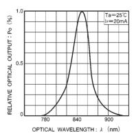
Fig. 3 Wavelength characteristics
