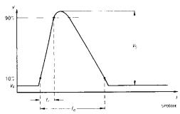
Parameters:  $V_S = 50 \text{ V (level II)}$   $V_P = 13.5 \text{ V}$   $R_i = 0.5 \text{ to } 4 \Omega$   $t_d = 40 \text{ to } 400 \text{ ms}$  $t_r = 0.1 \text{ to } 10 \text{ ms}$
