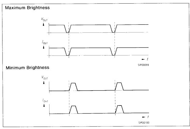
BTS 629 PWM Frequency characteristic min./max. Values
