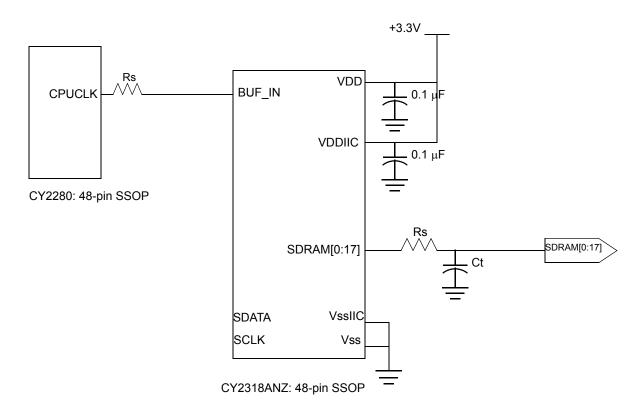
Rs = Series termination resistor Ct = Optional cap to reduce EMI
