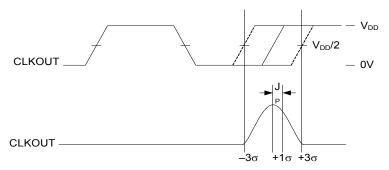
Figure 6. Cycle to Cycle Jitter
