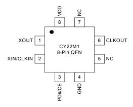
Table 1. Pin Definition: CY22M1 8-Pin 1.7 x 1.7 mm<sup>2</sup> QFN
