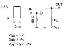
$\begin{array}{l} \text{Duty} \leq 1\% \\ \text{V}_{\text{IN}} : t_{\text{r}}, \, t_{\text{f}} < 5 \, \text{ns} \\ (Z_{\text{out}} = 50 \, \Omega) \\ \text{Common Source} \\ \text{Ta} = 25^{\circ}\text{C} \end{array}$
