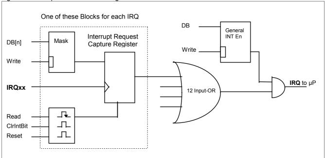
At power on or after any reset all interrupt request mask registers are cleared and therefore do not allow any interrupt request to be stored. Also the general interrupt enable **IntEn** is set to 0 (No IRQ to CPU) by reset.
