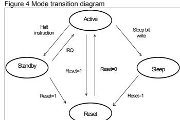
Due to the cold-start characteristics of the oscillator, waking up from sleep mode may take some time to guarantee stable oscillation. During sleep mode and the following start up the EM6520 is in reset state. Waking up from sleep mode clears the **Sleep** flag but not the **SleepEn** bit. Inspecting the **SleepEn** allows to determine if the EM6520 was powered up (**SleepEn** = "0") or woken from sleep mode (SleepEn = "1").
