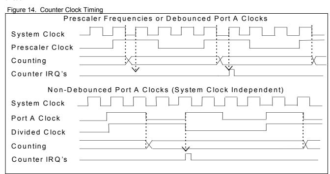
The two remaining clock sources are coming from the PA[0] or PA[3] terminals. Refer to the Figure 10 on page 14 for details. Both sources can be either debounced (Ck[11] or Ck[8]) or direct inputs, the input polarity can also be chosen. The output after the debouncer polarity selector is named PA3 , PA0 respectively. For the debouncer and input polarity selection refer to chapter 6.2.
