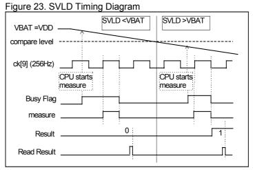
the power supply voltage was lower than the detection level value. During each read while **Busy=1** the **VLDResult** is not guaranteed.
