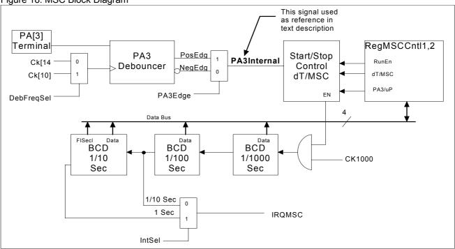
Changing **PA3Edge** while **RunEn=1** or **PA3/up=1** may generate a MSC event (start or stop). This behavior is useful for the - CPU controlled start and PA3 controlled stop - mode, But in general one does all the setup before starting the counter.
