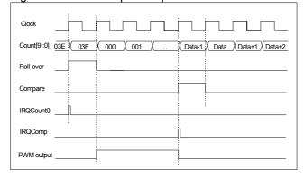
Figure 17. PWM Output in Down Count Mode
