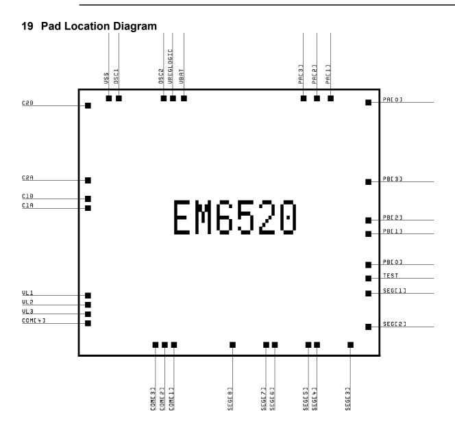
CHIP SIZE is X = 5232 by Y = 4648 Microns or X = 206 by Y = 183 Mils
