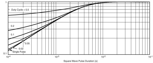
Normalized Thermal Transient Impedance, Junction-to-Case
