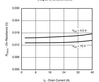
On-Resistance vs. Drain Current and Gate Voltage
