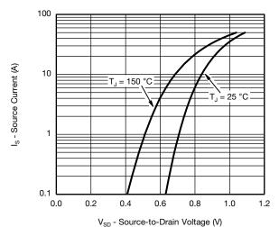
Source-Drain Diode Forward Voltage
