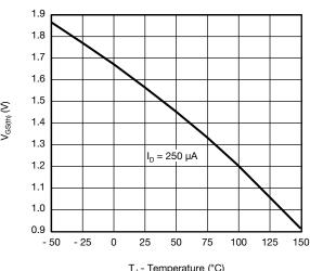
T<sub>J</sub> - Temperature (°C) **Threshold Voltage**
