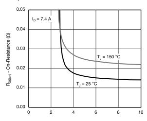
V<sub>GS</sub> - Gate-to-Source Voltage (V)
