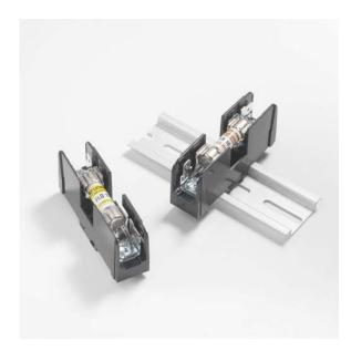
Littelfuse DIN series Class CC and Midget fuse blocks have integral DIN rail mounting capabilities that allow secure mounting to 35mm "hat" type DIN rails. Electrical panel builders and machine builders no longer need to use mounting adapters, saving assembly time and related costs. The blocks' interlocking feature allows multiple pole configurations to be created from single pole versions, in turn reducing the number of blocks in inventory.
