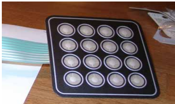
Figure 2. Low Cost Membrane Covered 4x4 Keypad that Interfaces to LCD+
