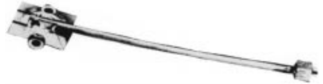
Figure 19. Photograph of 1/2" CQ Impedance Measurement Probe
