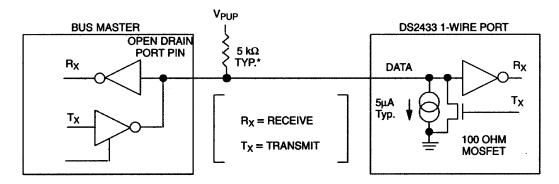
\* $5k\Omega$  is adequate for reading the DS2433. To write to a single device, a  $2.2k\Omega$  resistor and  $V_{PUP}$  of at least 4.0V is sufficient. For writing multiple DS2433s simultaneously or operation at low  $V_{PUP}$ , the resistor should be bypassed by a low-impedance pullup to  $V_{PUP}$  while the device copies the scratchpad to EEPROM.
