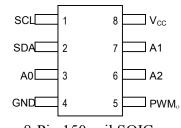
8-Pin 150-mil SOIC 8-Pin 118-mil μSOP
