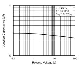
Fig. 5 - Typical Junction Capacitance
