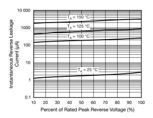
Fig. 4 - Typical Reverse Leakage Characteristics
