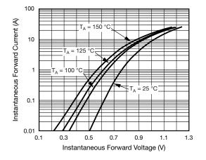
Fig. 3 - Typical Instantaneous Forward Characteristics
