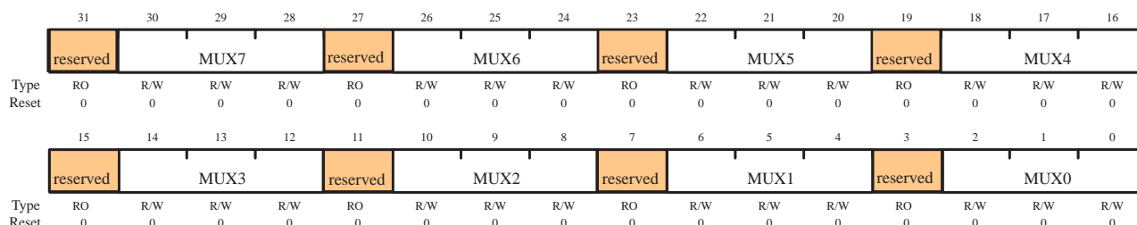
ADC Sample Sequence Input Multiplexer Select 0 (ADCSSMUX0)
